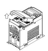
(3) Connect wires of WJ-VL to the control logic terminal.
